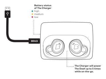
With The Dash in The Charger, connect to your computer or a power supply via USB.
